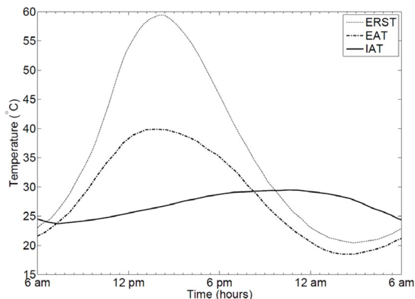
**Figure 3: External and internal air temperatures (EAT and IAT respectively) and external roof surface temperature (ERST) for a traditional adobe structure in Egypt (reproduced from Fitch (1960))**
