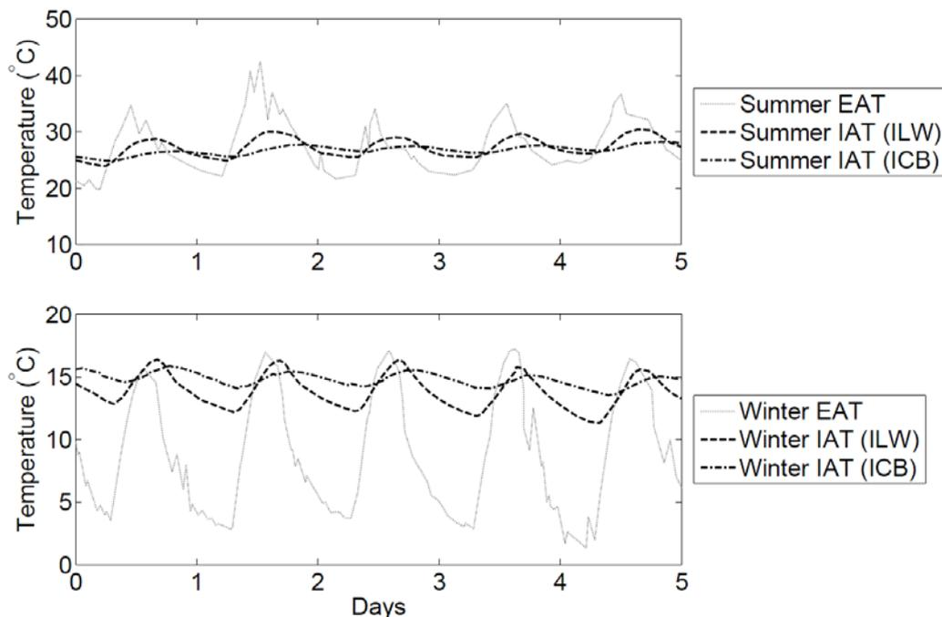
**Figure 2: External (E) and internal (I) air temperatures (AT) in ILW (high thermal resistance but low thermal mass) and ICB (low thermal resistance, high thermal mass) structures during typical summer and winter conditions (reproduced from Page *et al.* (2011)).**
